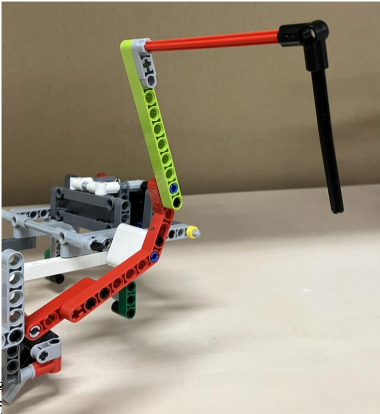
We added a solution to our robot that falls down when it enters the energy storage and thus brings two solar park energy to the base.
